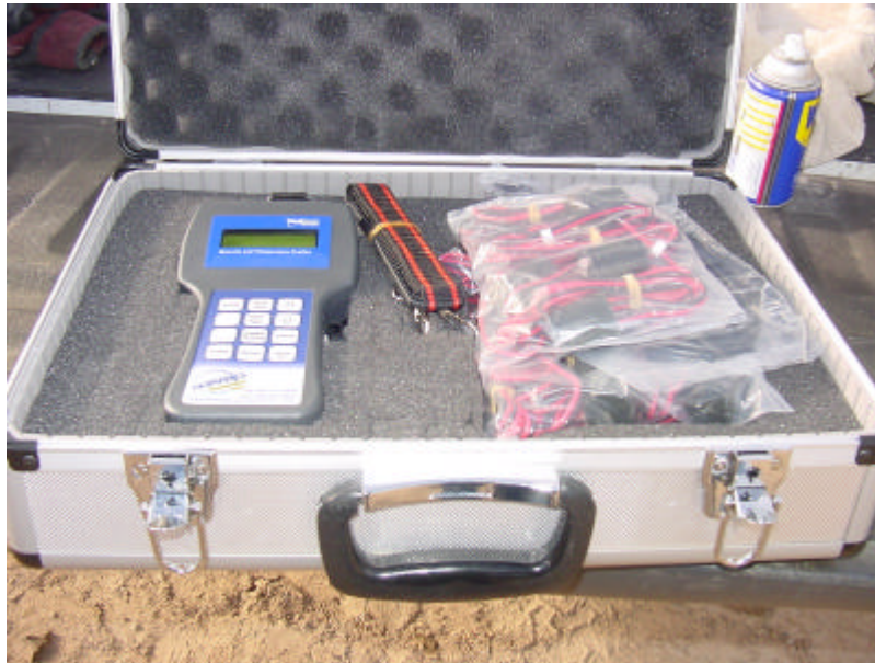
Figure 3. IntelliRock™ Maturity Reader and Maturity Loggers
