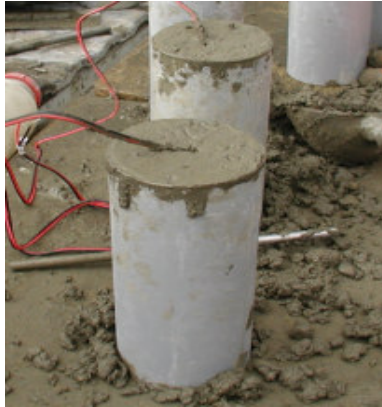
Figure 2.2 Cylinder specimens with embedded loggers
