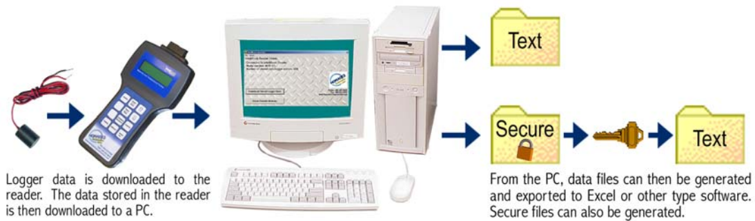
Figure 3-2 The Transferring process of the Logger data
